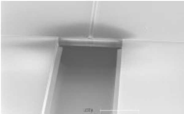
Figure 3: A SEM micrograph of a fibre guiding groove in front of a waveguide.
